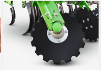
Levelling discs – with a particularly good self-driving effect
