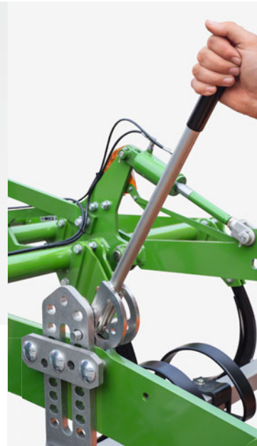
Manual adjustment of the levelling unit via the pin position
